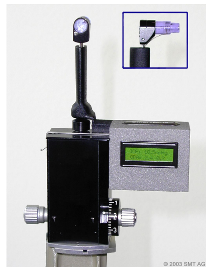
Fig. 3 Experimental DCT device. Custom-built contour tonometer tip is mounted on base of a Goldmann Tonometer, which is set to provide 1 gram appositional force. Pressure measured by sensor is read from LCD display and may be transmitted to a connected PC.
